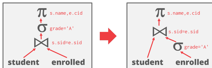
Figure 3: Predicate Pushdown: – Instead of performing the filter after the join, the filter can be applied earlier in order to pass fewer elements into the filter.
